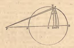
Draw E D, e d perpendiculars upon P S; let e d intersect E F in r; draw r n perpendicular upon E D. Then E r: n r:: P E: E D,  $\therefore$ E r. E D = n r. P S = D d. P E,  $\therefore$  the annular surface generated by the revolution of E r  $\alpha$  E r. E D  $\alpha$  D d. P E, and (P E remaining the same)  $\alpha$  D d. But the attraction of this annular surface on P  $\alpha$  D d. P E, and the attraction in the direction P E: the attraction in the direction P S:: P E: P D,
